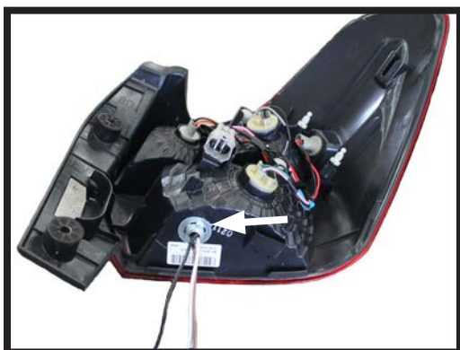
Drill a hole according to the tail light wiring kit instructions.
