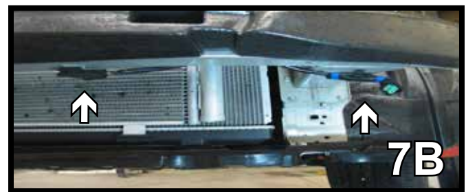
7. Disconnect wire connections from the right and left side of the bumper, as well as the sensors located underneath the bumper.
