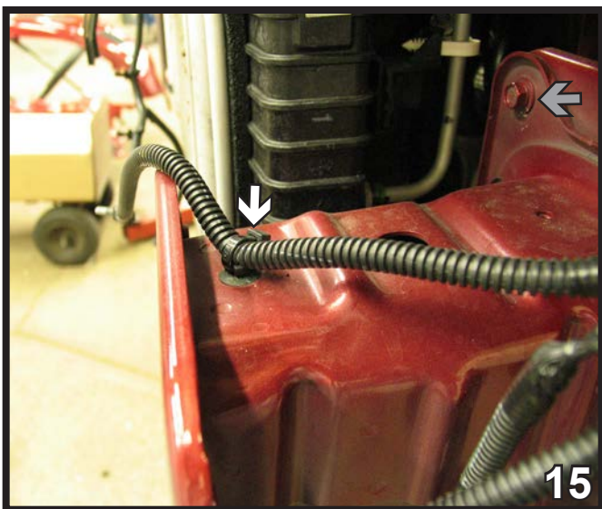
15. On the driver's side, remove the Christmas tree pin holding the wire loom. Pull wire loom out of the way.
