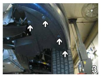
Remove four pushpins from the bottom edge of the fascia, just forward of the front tire. Set the pushpins aside to be reinstalled later. Do this to both sides of the vehicle. Pull fascia's upper corners out to the side of the vehicle and straight forward. Set the fascia aside carefully to be reinstalled later.
