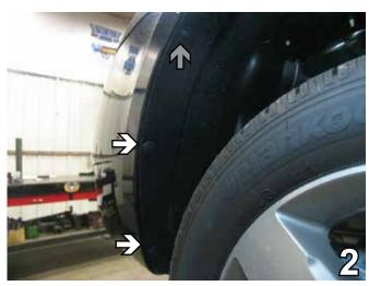
Using a 7MM socket, remove on metric bolt from just forward of the front tire on the edge of the wheel well cover. Set bolt aside to be reinstalled later. Remove two pushpins from the same location. Set pushpins aside to be reinstalled later. Do this to both sides of the vehicle.
