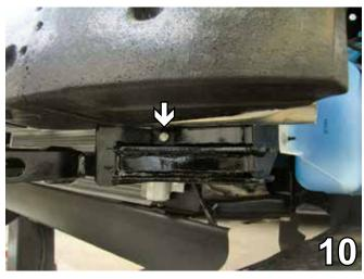
10. Using the baseplate as a template, drill the hole just below the metal bumper with the 13/32" drill bit. Do this to both sides of the vehicle. Insert the 3/8" hex bolt into the drilled hole, tighten the 3/8" hex nut and lock washer on the back side of the bumper bracket webbing. Do this to both sides of the vehicle.
