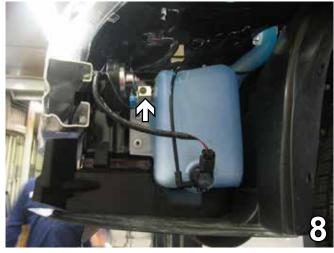
8. Using a 10MM socket, remove one metric bolt from the horn bracket on the driver's side. Unplug the electrical connections. Set the horn bracket and the metric bolt aside to be reinstalled later.
