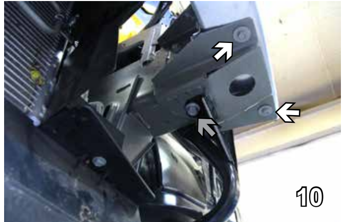
10. Remove three bolts underneath the bumper. Use a 10MM socket on the top two and a 15MM socket for the bottom one (grey arrow). Set aside bolts for later reinstallation.
