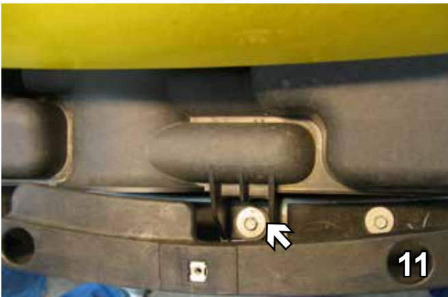
11. Up on top, remove one bolt using a 10MM socket. Set aside bolt for later reinstallation.
