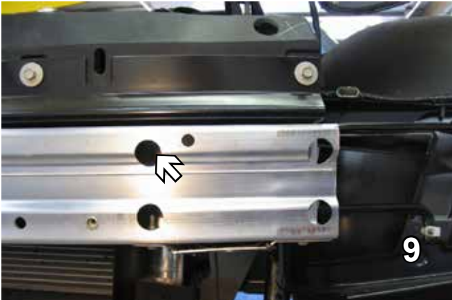
9. Using a 13MM socket, remove two more bolts from both sides. Set bolts aside to be reinstalled later.
