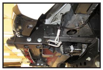
13. Attach the permanent baseplate safety cables to the provided convenience link on the baseplate. The photo above shows the recommended installation of the cables to frame of vehicle. Additional options may interfere with suggested mounting; in this case, secure the cables to a solid piece of the frame as described in the General Information sheet. Be sure the safety cables do not rub against any hoses or moving parts. Do this on **BOTH** sides of the vehicle.
