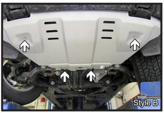
6. Using a 15MM socket, remove the front two (2) bolts of the belly pan. Loosen the back two (2) bolts then slide belly pan off and set aside to be reinstalled later.
