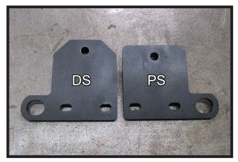
8. There are two (2) support brackets styles for each side of the vehicle. The tapered edge brackets are for the driver side of the vehicle and the square edge brackets are for the passenger side of the vehicle. Note: The plates with the welded spacer are installed toward the inside of the vehicle.
