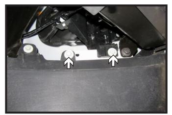
4. **For Vehicles with a Shroud:** Using a 10MM socket, remove the two (2) bolts from the underside of the vehicle. Do this on both sides of the vehicle.
