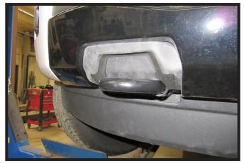
1. Remove plastic shield from both tow hooks.
