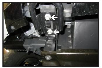
Using a 15MM socket, remove the two (2) bolts from the tow hook. Remove tow hook, it will not be reinstalled. Do this on both sides of the vehicle.
