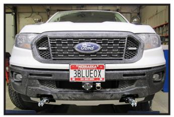
15. **For Vehicles with a Shroud:** Hold shroud up to the vehicle, as close to the original position as possible. Mark and trim as needed to allow clearance for baseplate. Reinstall plastic shroud.
