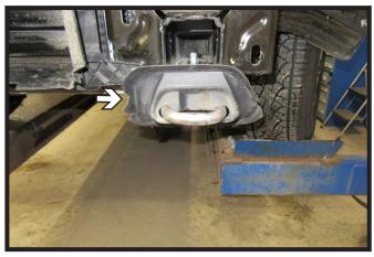
3. Remove the rubber piece from the tow hook. Do this on both sides of the vehicle.
