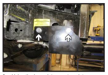
6. Using the baseplate as a template, use a 1/2" drill bit to drill two (2) holes through the frame of the vehicle. Install two (2) 1/2" bolts with hardware. Do this on both sides of the vehicle.
