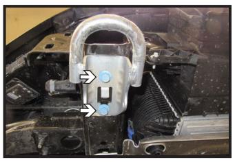
Using a 15MM socket, remove the two (2) bottom bolts from the tow hook. Remove tow hook and set aside, it will not be reinstalled. Do this on both sides of the vehicle.
