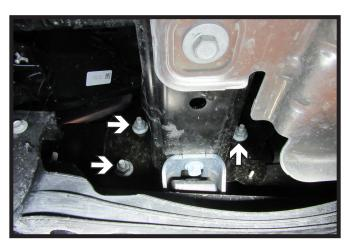
Using a 21MM socket, remove the three
