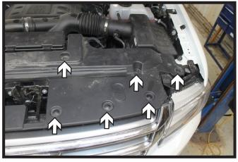
1. Using a Phillips screwdriver, remove the twelve (12) push pins from the top edge of the fascia cover. There are six (6) on each side. Set the cover aside.
