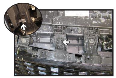
7. Unsnap the fascia by the headlight locations (inset). Lift piece over the two (2) hooks on the top of the fascia. Pull the corners of the fascia away from the vehicle disconnecting any electrical connections and set the fascia aside to be reinstalled later.
