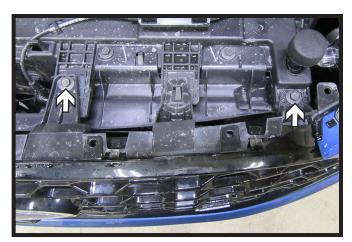
Using a 10MM socket, remove the four (4) bolts from the top edge of the fascia. There are two (2) on each side.
