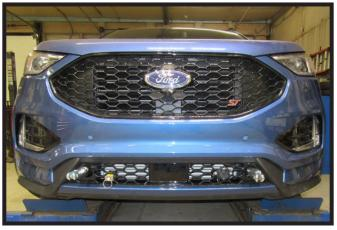
20. Hold the fascia as close to its original position, mark and trim the fascia around the convenience links and attachment tabs. Reinstall the fascia, fascia cover, and headlights.
