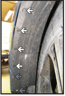
Using a 5.5MM socket, remove the four
