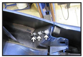
4. Using an 8MM socket, remove the three (3) bolts from the fascia/fender joint underneath where the headlight was. Do this on both sides of the vehicle.
