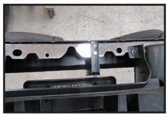
14. **Optional:** On the backside of the fascia there are two (2) existing holes above the license plate, use either hole to attach the bracket for the breakaway switch.
