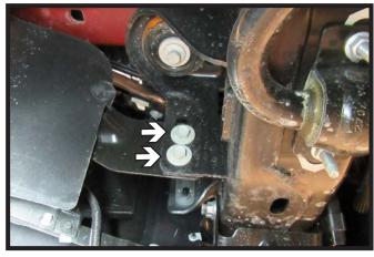
2. Behind the bumper on the frame by the headlights there are two (2) bolts that need to be removed using a 15MM socket, do this on both sides of the vehicle.
