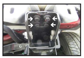
Using an 18MM socket, remove the four
