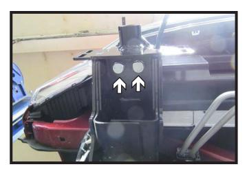
11. Slide the baseplate on, align with the existing front tow hook holes. Bolt on first using two (2) of the 5/8" x 1-3/4" bolts, and lock washers.
