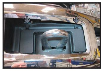
Remove the two (2) clips from each side above the tow hook. Do this on both sides of the vehicle.
