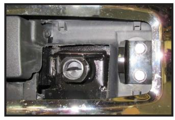
18. Trim the tow hook bolt cover as shown before reinstalling to allow room for the convenience link (left). Do this for both sides of the vehicle. **Note:** For vehicles with ACC, do not reinstall the bolt cover on the driver side of the vehicle (right).
