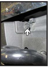
4. Models with Adaptive Cruise Control (ACC): Using a 10MM socket, remove the two (2) bolts from the cover of the ACC on the driver side of the vehicle.
