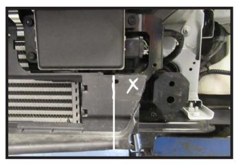
11. Using a utility knife remove the indicated area on the driver side of the vehicle.
