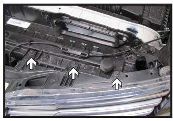
Using a 10MM socket remove the three
