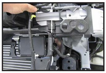
On the driver side of the vehicle remove the wiring harness from the push pin bracket. Using a utility knife remove the indicated areas.
