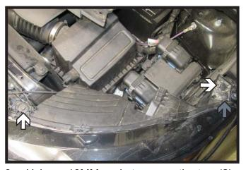
3. Using a 10MM socket remove the two (2) bolts (white) and one (1) push pin (gray) from the top of the headlight. Disconnect all electrical connections and set headlight aside. Do this on both sides of the vehicle.
