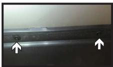
6. Using a 5.5MM socket, remove the eighteen (18) screws from the underside of the fascia. There are eight (8) on each side and two (2) in the center.
