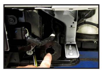
17. Using a 1-1/4" drill bit drill one (1) hole as indicated. Do this on both sides of the vehicle.
