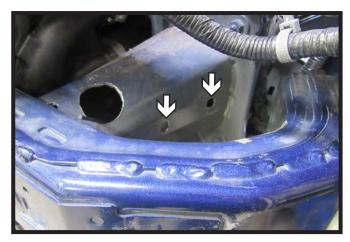
14. Using a 3/8" drill bit, ream out the rear existing hole. Do this on both sides of the vehicle.
