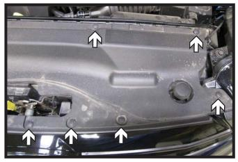
Remove the twelve (12) push pins along the top of the fascia cover. Set fascia cover aside to be reinstalled later.
