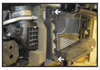
Remove the two (2) push pins and then remove the back plastic piece to allow baseplate to fit.
