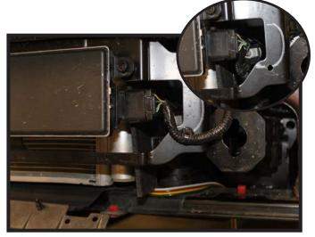
8b. **ACC Models:** Disconnect the ACC sensor wiring loom and re-route it in behind the metal framing to protect it from rubbing on the baseplate.
