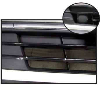
25. Optional: If there is an electrical plug for the engine block heater on the passenger side of the vehicle the following piece will need to be removed from the grill area as indicated.
