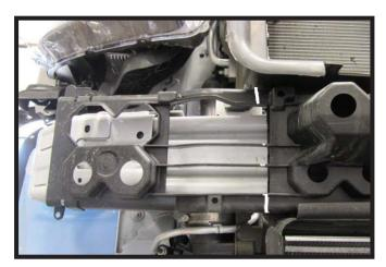
13. Using a utility knife remove the indicated areas on the passenger side of the vehicle.
