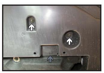
7. Using a 7MM socket remove the two (2) bolts (white) and one (1) push pin (gray) from the belly pan. Do this on both sides of the vehicle. Remove belly pan.
