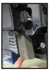
15. Remove the indicated foam pieces from both sides of the vehicle.
