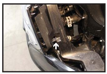
7a. Unsnap the fascia by the headlight locations. Pull the corners of the fascia away from the vehicle disconnecting any electrical connections and set the fascia aside.
