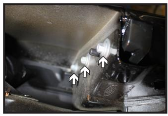
5. Using a 8MM socket, remove the three (3) bolts from the fascia/fender joint underneath where the headlight was. Do this on both sides of the vehicle.
