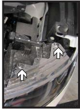
2. Using a T25 Torx, remove the four (4) screws from above the headlights. There are two (2) on each side.
