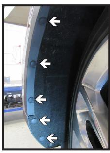
4. Remove the five (5) push pins from along the edge of the wheel well. Do this on both sides of the vehicle.
