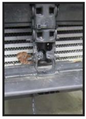
11. Trim the shutter housing on both sides of the vehicle and in the middle as shown to allow room for the baseplate cross member.
