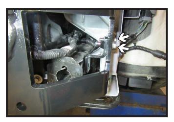
19. Using two (2) 3/8" bolts attach the Z bracket to the side plate as indicated.
