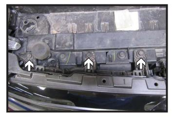
Using a 10MM socket, remove the six (6) bolts from the top of the fascia. There are three (3) on each side.
