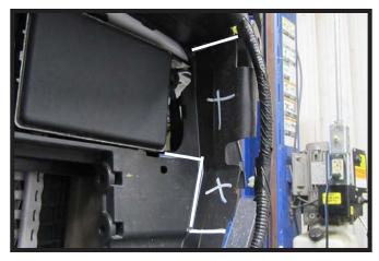
9. Using a utility knife remove the indicated areas on the driver side of the vehicle.
