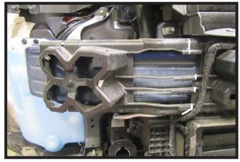
12. Using a reciprocating saw, cut the corner plastic piece off of the driver and passenger side where marked and remove plastic piece.
