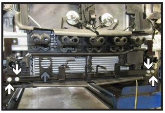
20. Using four (4) 1/2" x 2-3/4" bolts with lock washer and nylon lock nut attach the center cross bar to the side plates. If the holes do not completely line up, ream out holes with a drill bit.
