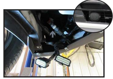
8. Unplug electrical cable on the underside of the fascia. If the vehicle has a plug on the passenger side of the vehicle as shown in insert, will need to unplug the engine bock heater as indicated (gray) and remove. Then remove the fascia.
