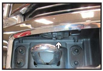
On the passenger side of the vehicle pull the indicated plug through the backside of the fascia and let hang. Pull the bumper forward and set aside to be reinstalled later.
