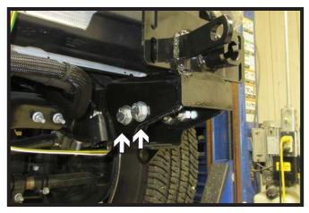
11. Use three (3) 1-3/4" bolts to attach the baseplate towards the outside of the frame. Use a flat washer on the outside and nylock nut on the inside for the front two (2) bolts indicated with a white arrows and a flat washer and nylock nut on the inside for the third bolt indicated with a gray arrow. Towards the inside of the frame use two (2) 1-3/4" bolts to attache the baseplate with the washer on the outside and nylock nut on the inside. Do this on both sides of the vehicle.
