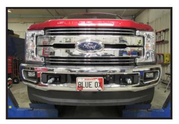
14. Reinstall bumper, bolts, and reconnect wiring.
