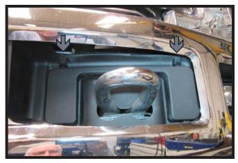
3. Remove the two (2) clips from each side above the tow hook. Do this on both sides of the vehicle.
