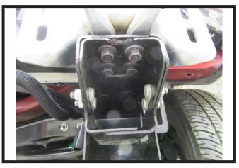
Using an 18MM socket remove the four
