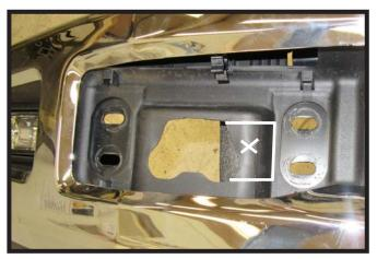
12. Using a reciprocating saw remove the marked area on both sides of the fascia towards the inside near the licence plate.
