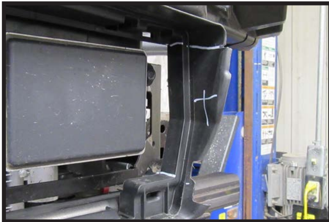
13. Using a reciprocating saw, trim the marked area on the driver's side shutter.
