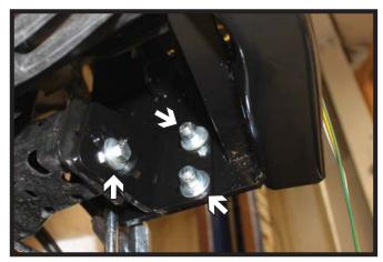
12. Install the support plate to the lower two (2) baseplate holes and the existing hole on the face of the frame horn with the 3/8" hardware. Fully tighten all fasteners. Do this on both sides of the vehicle.
