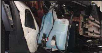
14. Install nine (9) 1/4" washers onto the two (2) studs for the washers reservoir (top). Reinstall the washer reservoir onto the studs and reinstall the factory nuts. The factory screw will not be reinstalled.
