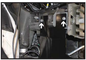
11. Using a 3/8" drill bit, drill the upper two (2) holes on the side of the baseplate thru the frame. Install the 3/8" hardware and fully tighten. Do this on both sides of the vehicle.
