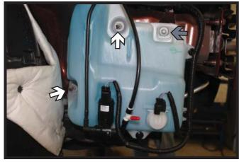
6. Using a 11MM socket, remove the two (2) nuts from the washer reservoir (white). Then using a 8MM socket, remove the screw (gray). Disconnect/plug all lines and set the reservoir aside.
