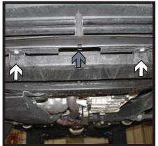
8. **Shutter Models Only:** On the driver side, remove the two (2) screws from the shutter motor and unsnap from the housing (left).
