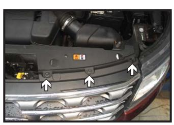
Using a 10MM socket, remove the seven (7) screws from the top edge of the fascia. There are three (3) on the driver side and four (4) on the passenger side.
