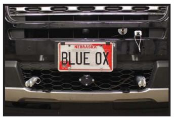
16. Hold the fascia as close to its original position, mark and trim the fascia around the convenience links and attachment tabs. Reinstall the fascia.
