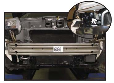
10. Install the baseplate onto the frame and clamp in place. Install the 3/4" bolt and lock washer into the existing hole on the under side of the frame (inset). Insert the 3/4" nut plate on the inside of the frame, level the baseplate and fully tighten the bolt. Do this on both sides of the vehicle.
