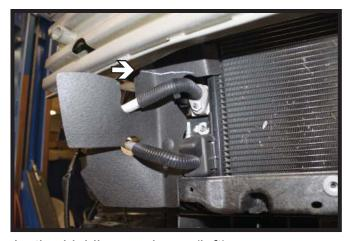
7. **Non ACC models:** On the driver side, trim the plastic shielding as shown (left). **EcoBoost Models:** On the passenger, trim the plastic shielding as shown (right).
