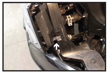
6. Unsnap the fascia by the headlight locations. Pull the corners of the fascia away from the vehicle disconnecting any electrical connections and set the fascia aside.
