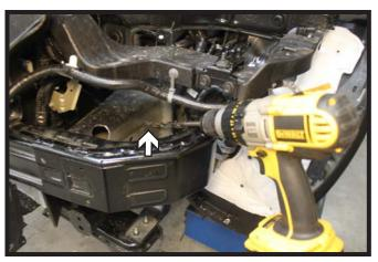
10. Using a 3/8" drill bit, ream out the rear existing hole. Do this on both sides of the vehicle.
