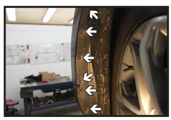
5. Using a 5.5MM socket, remove the six (6) screws from the edge of the wheel well. Do this on both sides of the vehicle.
