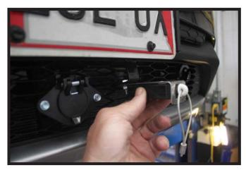
18. **Optional Breakaway:** The breakaway bracket can be installed to the license plate bracket or the lip of the fascia at the desired location with the supplied 1/4" hardware.
