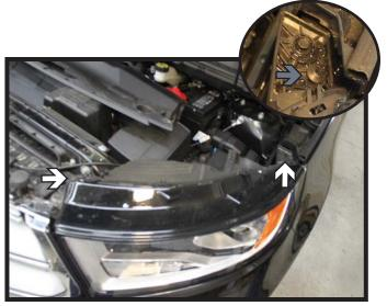
3. Using a 10MM socket, remove the two (2) screws from the headlight (white). Remove the indicated push pin from the driver side (gray). Disconnect all electrical connections and set the headlight aside. Do this on both sides of the vehicle.
