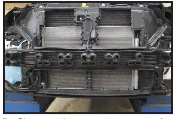
7. Disconnect the temperature sensor and wiring loom from the plastic bumper cover. Unsnap the bumper cover from the bumper and set aside.
