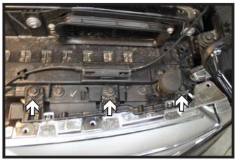
2. Using a 10MM socket, remove the six (6) screws from the top edge of the fascia. There are three (3) on each side.
