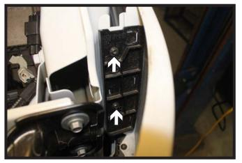
Underneath where the headlight was, using a T25 Torx, remove the two (2) screws from the fascia/fender joint. Do this on both sides of the vehicle.
