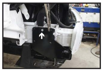
14. Install the baseplate onto the frame, flushing it to the top of the frame. Clamp into place and drill the middle hole thru the frame with a 3/8" drill bit. Install a 3/8" bolt with lock washer into the hole with a 3/8" whiz nut on the inside of the frame lip. Do this on both sides of the vehicle. Level the baseplate and fully tighten the all hardware.
