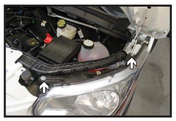
2. Using a T30 Torx, remove the two (2) screws from the headlight. Disconnect any electrical connections and set aside. Do this on both sides of the vehicle.
