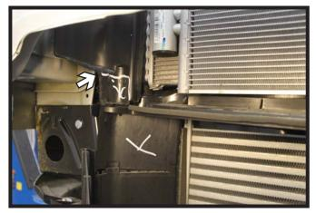
Trim the upper section of sheilding just below the bumper and disconnect the lower section. Do this on both sides of the vehicle.
