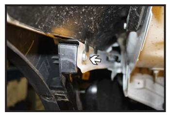
5. Pull back the fender flare and using a 10MM socket, remove the screw from the inside of the fascia/fender joint. Do this on both sides of the vehicle.
