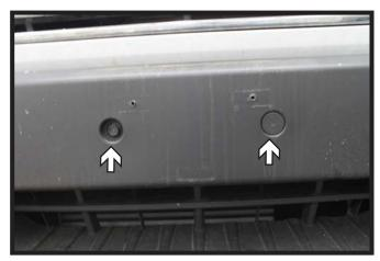
8. Remove the plugs from the fascia. Then using a 13MM socket remove the two (2) screws from the face of the fascia.
