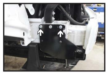
15. Continue drilling the remaing top holes thru the frame with a 3/8" drill bit. Installing 3/8" bolts with lock washers into the holes with a 3/8" whiz nuts on the inside of the frame lip. Do this on both sides of the vehicle. Fully tighten the all hardware.
