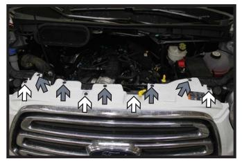
Using a 10MM socket, remove the four (4) screws from the top edge of the fascia (white). Then remove the five (5) push pins (gray).
