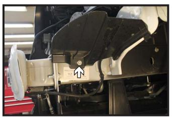
On the driver side, using a 10MM socket, remove the screw from the plastic shield. The sheild will not be reinstalled.
