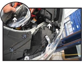
2. On the top side of the fascia, remove the two (2) push pins (gray). Then using a T25 Torx remove the two (2) screws from the headlight assembly (white). The second screw is underneath the cover (inset).
