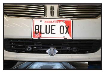
15. Hold the fascia as close to its original position, mark and trim the fascia around the convenience links and attachment tabs. Important: Ensure that nothing is installed in front of the ACC sensor. Obstructions will cause false readings from the sensor. Reinstall the fascia.
