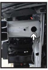
9. Using a 1-1/4" hole saw, drill an access hole on the passenger side (left) and driver side (right) as shown for nut plate access.
