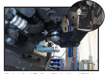
12. Install a 1/2"-13 x 4" bolt with a 1/2" flat washer into the bottom hole (white). Use four (4) to five (5) 1/2" washers in between the baseplate and extension as shims (gray). Install a 1/2" flat washer, 1/2" lock washer and 1/2" hex nut onto the bolt on the top side of the extension (inset). Do this on both sides of the vehicle. Level the baseplate and tighten down all hardware.
