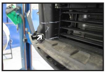
6. Trim the radiator shrouding approximately as shown for baseplate clearance. Do this on both sides of the vehicle.
