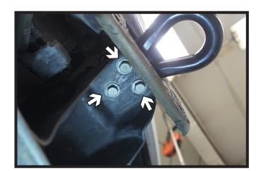
Using a 15MM socket, remove the six (6) bolts from the tow hooks. There are three (3) on each side. The tow hooks will not be reinstalled.
