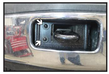
1. Using a 13MM socket, remove the two (2) bolts from wheel well. There is one (1) on each side (left). Then using a 18MM socket, remove the four (4) bolts from face of the bumper. There is two (2) on each side (right). Set the bumper aside.
