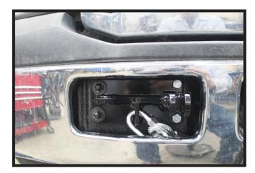
cables to the provided convenience link on the baseplate. The photo above shows the recommended installation of the cables to frame of vehicle. Additional options may interfere with suggested mounting; in this case, secure the cables to a solid piece of the frame as described in the instructions included with the permanent baseplate safety cables. Be sure the safety cables do not rub against any hoses or moving parts. Do this on **BOTH** sides of the vehicle.
