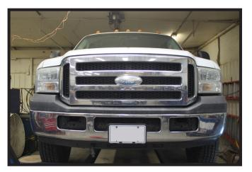
Reinstall the bumper to the vehicle. Using only the wheel well bolts and passenger side face bolts. The driver side bolts will remain out during the baseplate installation.
