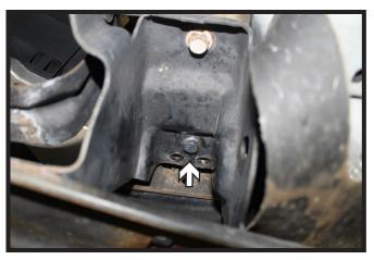
4. Insert the DS baseplate into the frame, start a 1/2"-13 x 1-3/4" bolt with 1/2" lock washer into the bottom rear tow hook hole and finger tighten (right). Reinstall the two (2) existing bumper bolts (left) and fully tighten all three bolts.
