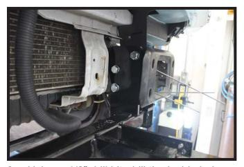
Using a 1/2" drill bit, drill the inside holes thru the frame on each frame rail. Install a 1/2"-13 x 1-1/2" bolts with a 1/2" lock washers into the holes and secure with 1/2" nut plates on the inside of the frame. Fully tighten all fasteners.
