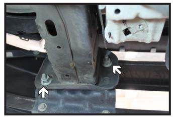
Using a 21MM socket, remove the four (4) nuts from the inside of the bumper. There are two (2) on each side. Set the bumper aside.
