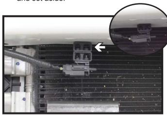
7. On the passenger's side, unclip the air temperature sensor from the bumper.
