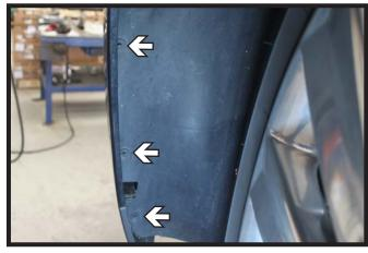
Using a 5.5MM socket, remove the three
