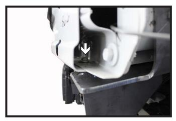
10. On the driver side bumper, using a chisel or flat screwdriver, remove the nut welded on the inside of the bumper for bolt clearance on step #13.
