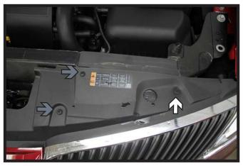
Using a 10MM socket, remove one (1) bolt from the top of the fascia (white).
