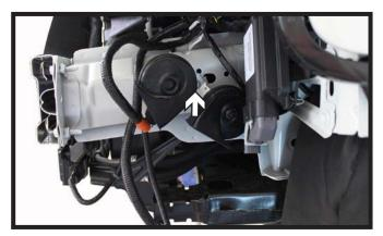
On the driver side, using a 8MM socket, remove one (1) bolt from the horn bracket and set aside.
