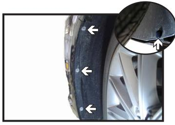
3. Using a 5.5MM socket, remove the three (3) screws from the outer edge of the wheel well. Then on the inner lower edge of the wheel well, remove the one (1) push pin (inset). Do this on both sides of the vehicle.
