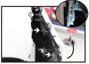
4. Pull back the wheel well liner, then using a 10MM socket, remove the three (3) nuts from inside of the fender. Then pull the corner of the fascia outward and forward. Do this on both sides of the vehicle. Disconnect all electrical connections and set the fascia aside.
