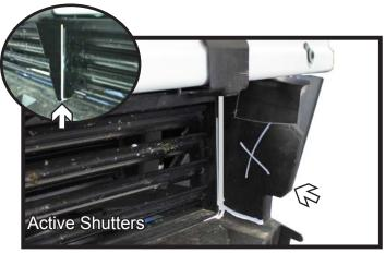
8. **Non-Active Shutters:** Trim the plastic shrouding off just below the bumper as shown for baseplate clearance. Do this on both sides of the vehicle.
