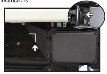
9. **Adaptive Cruise Control Models:** On the driver side, install the support bracket onto the bumper and ACC sensor bracket as shown. Mark and drill the holes with a 1/4" drill bit. Attach the bracket with 1/4"-20 x 3/4" bolts and 1/4"-20 lock nuts. Once the bracket is installed, use a reciprocating saw to remove the outer edge of the ACC bracket (inset).
