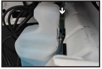
15. Reinstall the washer reservoir to the vehicle, using seven (7) 1/4" flat washers as a spacer on the top back hole to keep the reservoir from rubbing on the baseplate.
