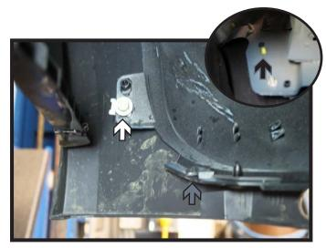
4. Using a 10MM socket, remove the screw from the inside corner of the fascia (white). Then release the clip below (gray). Further up on the inside of the fascia above the screw, release the yellow clip holding on the fender flare (black). Do this on both sides of the vehicle.
