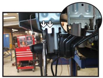
Bend the first two (2) tabs of the frame back at a 90° angle for baseplate clearance. Do this on both sides of the vehicle.
