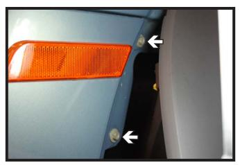
5. Pull the fender flare away the vehicle. Then using a 10MM socket, remove the two (2) screws from the behind the fender flare. Do this on both sides of the vehicle.
