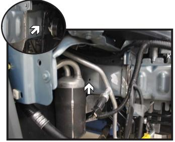
9. Using a 13/32" drill bit, drill out the existing hole in the frame. Do this on both sides of the vehicle.
