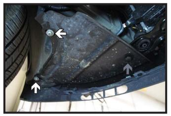
3. On the underside of the fascia on the driver side only, using a T30 Torx, remove the two (2) screws (white). Then remove the push pin (gray).
