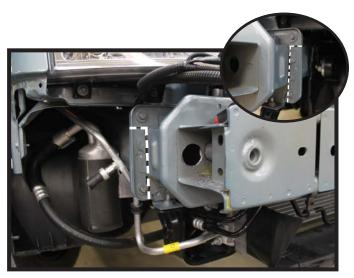
8. Using a reciprocating saw, trim the frame extension on both the driver and passenger sides as shown.
