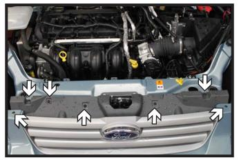
1. Using a Phillips screwdriver, remove the seven (7) screws from the top edge of the fascia.
