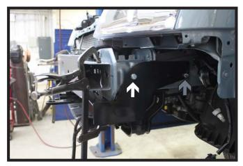
12. Position the baseplate onto the vehicle, temporarily pinning the back holes with a 3/8" bolt (gray). Level and clamp the baseplate into position. Using a 13/32" drill bit, drill the front hole thru the frame. Install a 3/8"-16 x 1-1/2" bolt with a 3/8" lock washer into the hole and a 3/8" nut plate on the inside of the frame (white). Do this on both sides of the vehicle. Tighten both fasteners down.
