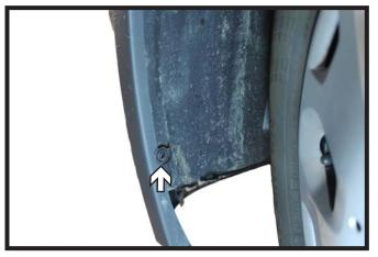
2. Using a Philips screwdriver, remove the screw from the outer edge of the wheel well. Do this on both sides of the vehicle.
