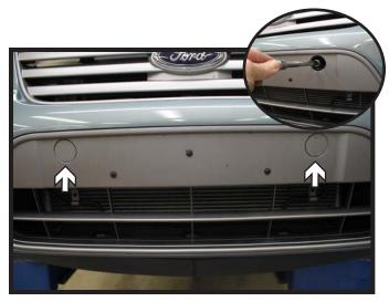
6. Remove the two (2) plastic covers. Then using a T40 Torx, remove the two (2) screws from the fascia. Remove the fascia from the vehicle and set aside.
