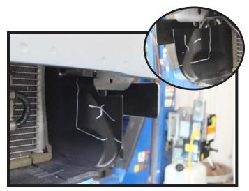
10. Trim the air shrouds on both sides of the vehicle as shown for baseplate clearance.
