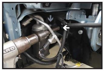
13. Using a 13/32" drill bit, drill the middle hole thru the frame. Install a 3/8"-16 x 1-1/2" bolt with a 3/8" lock washer into the hole and a 3/8" nut plate on the inside of the frame (white). Remove the back bolt, ream out the hole if necessary, reinstall the bolt with a 3/8" lock washer and a 3/8" nut plate on the inside of the frame (gray). Do this on both sides of the vehicle. Tighten all fasteners down.
