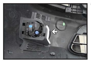
15. On the backside of the fascia, trim the edge of the fog lamp housing as shown. Do this on both sides of the fascia. Reinstall the fascia and plastic covers.
