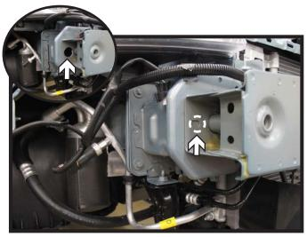
7. On the passenger side only, using a 1-1/4" hole saw, drill an access hole into the frame extension.
