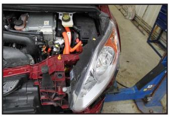
12. Plug in and reinstall the headlights on both the driver and passenger sides. Secure any loose wiring.
