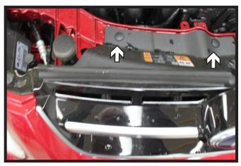
Remove the two (2) push pins from the top back edge of the fascia. Do this on both sides of vehicle.
