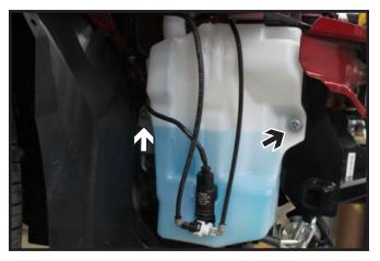
15. On the passenger side, reinstall the washer fluid reservoir. Reuse one (1) of the existing screws on left side (white). Then a 3/8"-16 x 1" bolt, 3/8" flat washer and 3/8" lock nut on the right side (black).
