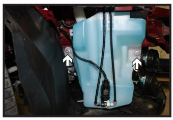
On the passenger side, using a 10MM socket, remove the two (2) screws from the washer fluid reservoir. Disconnect lines and set reservoir aside.
