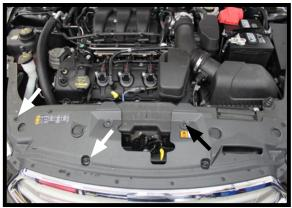
1. Using a 10MM socket, remove the four (4) bolts, two (2) per side. Use a flat screwdriver to pry the push pin out. There are two (2) located toward the center of the vehicle.
