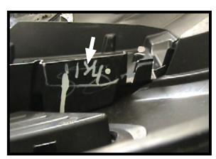
21. Measure down 1-1/4" and all the way over to the outer edge on the backside of the front fascia. Notch this as shown to allow for proper clearance.
