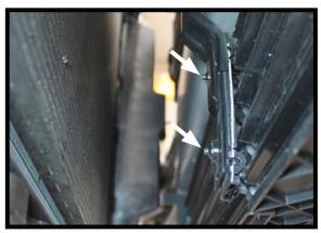
On the backside of the air shutter there are three (3) clamps. Tightly squeeze the clamp button to release. There are three (3) buttons on each clamp, two (2) towards the bottom and one (1) towards the top.
