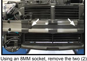
8. Using an 8MM socket, remove the two (2) bolts. Unclip the air temperature sensor and place to the side.
