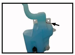
16. Prior to reinstalling the windshield wiper fluid reservoir, notch as shown above.
