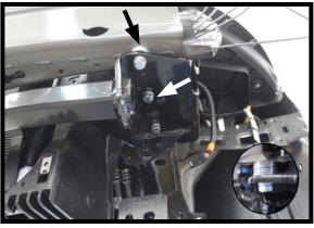
14. Drill the three (3) bottom holes using a 13/32" drill bit.
