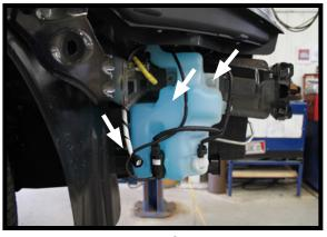
10. The windshield wiper fluid reservior needs to be removed on the passenger side. Unplug all electrical components and remove the bolts. On the top, right side, remove the bolt using an 8MM socket. The other two (2) bolts require a 11MM socket for removal.
