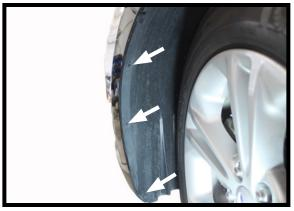
2. Remove the three (3) bolts located on the outer edge of the wheel well area with a 5.5MM socket. Do this on both sides of the vehicle.
