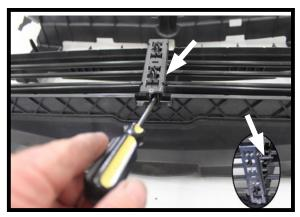
19. Lay the air shutter on a flat, sturdy surface. Insert a flat screwdriver into the top portion of the air shutter bracket and pop up. Do the same on the bottom portion.
