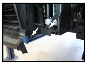
7. Use a flat screwdriver to remove the two (2) push pins on the air dam support brackets. These brackets are located on the side of the air dam.
