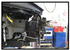
13. Drill one (1) hole using a 13/32" drill bit. Do this on both sides of the vehicle. Recheck the baseplate for proper alignment. After making any adjustments necessary, drill the second hole on each side.
