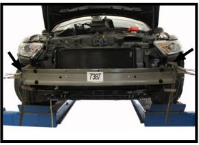
12. Clamp the baseplate securely into place and verify it is properly aligned.
