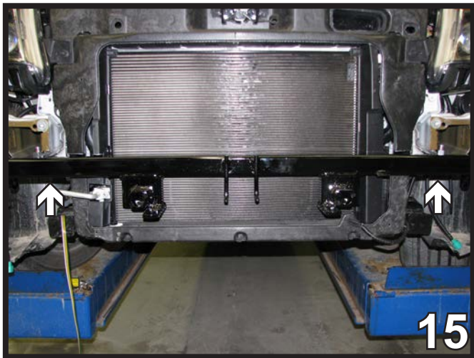
15. Tip the baseplate up, lower the driver's side down, slide the baseplate in, lift up and clamp. Start the 3/4-10 bolt in the frame bottom existing hole. Do this on both sides.
