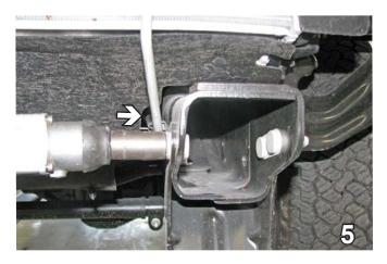
5. On the driver's side, it will be necessary to pull the Christmas tree pin from the coolant line bracket that goes into the frame in order to position the baseplate. It will be reinstalled later.
