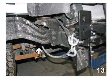
13. Attach the permanent baseplate safety cables to the provided convenience link on the baseplate. The photo shows the recommended installation of the cables to frame of vehicle. Additional options may interfere with suggested mounting; in this case, secure the cables to a solid piece of the frame as described in the General Information sheet. Be sure the safety cables do not rub against any hoses or moving parts. Do this on BOTH sides of the vehicle.
