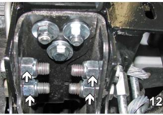
Slide the lower support bumper brace (removed in step 7) over the baseplate to align with the reamed holes. The brace may need to be widened to fit. Tighten all four 5/8-11 x 2" bolts attached to 5/8-11 hex nuts on the inside. Use Loctite Red on all bolts. Do this on both sides.
