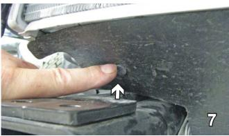
On the passenger side, on the back bottom of the lower radiator, remove the push pin from the rubber air dam. Set the pin and the air dam aside to be reinstalled later.
