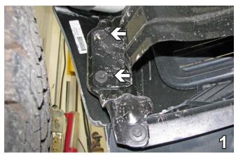
1. Using a 13MM socket, remove two metric bolts located just forward of the front tire. Do this to both sides of the vehicle. Set bolts aside to be reinstalled later.
