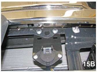
15. Install 1/4-20 x 3/4" bolts with 1/4" flat washers, 1/4" lock washers and 1/4-20 whiz nuts. Reinstall the air dam, coolant transfer box, Christmas tree pins, heat core plug, bumper, cover, push pins, bolts and reconnect wiring.
