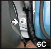
6. On the passenger side using an 8MM socket, remove one bolt from the top of the washer reservoir. Using a 10MM socket, remove two bolts one on each side. Disconnect the electrical connections and the hoses and remove the washer reservoir. Cap the fluid openings. Set the washer reservoir and bolts aside to be reinstalled later.
