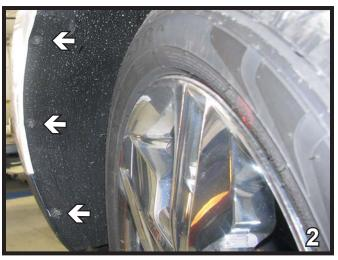
Using a 5.5MM socket, remove three bolts just forward of the front tire on the wheel well. Do this to both sides of the vehicle. Set bolts aside to be reinstalled later.
