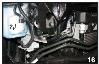
16. On the passenger side, reinstall the washer reservoir. Reconnect the electrical connections and the hoses.
