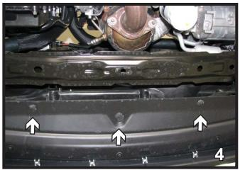
4. Using a flat screwdriver, remove three push pins across the middle. Set push pins aside to be reinstalled later. Pull the fascia up and out to remove from the vehicle and set aside carefully to be reinstalled later.
