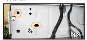
12. Using a 1 1/4" hole saw, drill two 1 1/4" holes into the frame, so an extension can be used to tighten up bolts. Do this to both sides of the vehicle.
