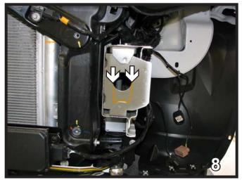
On the front of the frame, using a reciprocating saw, cut straight down on the dashed lines. Bend in across the bottom. Do this to both sides of the vehicle.
