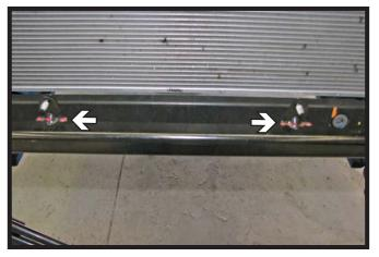
10. Using a reciprocating saw, cut off the tabs that the lower coolant line were attached to, being careful not to cut into the radiator.
