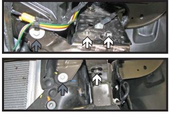
6. Using a 13MM socket, remove the two (2) bolts from the top of the metal bumper and one (1) bolt from the bottom (white). Then using a 10MM socket, remove the one (1) bolt from the top and bottom of the bumper (gray). Do this to both sides of the vehicle. Remove the metal bumper from the vehicle, the bumper will not be reinstalled later.
