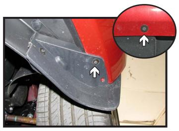
4. **2011-13 Models:** Using a 5.5MM socket, remove the three (3) screws from the underside of the fascia. There is one (1) in each corner and one (1) in the middle.
