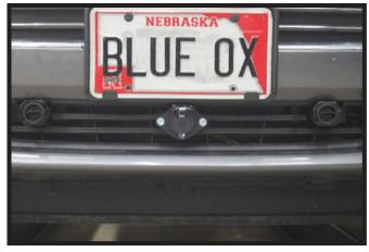
19. Reinstall the headlights. Hold the fascia as close to its original position, mark and trim the fascia around the convenience links and attachment tabs. Reinstall the fascia.
