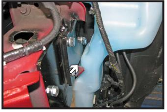
17. Reinstall the washer reservoir. Checking the clearance on the lower part of the reservoir making sure it is not rubbing on the baseplate. It should have minimum 1/16" clearance. If necessary pull the reservoir back and re-tighten the bolts.
