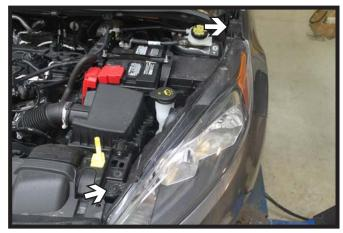
5. **2014 Models:** Using a T30 Torx, remove the two (2) screws from the headlight. Disconnect the electrical line and set the head light aside. Do this on both sides of the vehicle.
