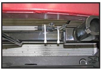
2011-13 Models: Attach the temperature sensor to the baseplate crosstube with zip ties.
