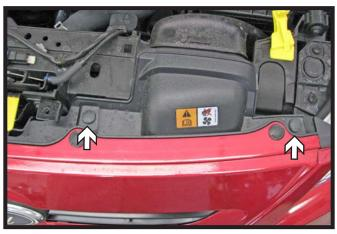
1. **2011-13 Models:** Remove the four (4) push pins from the top edge of the fascia. There are two (2) on each side.
