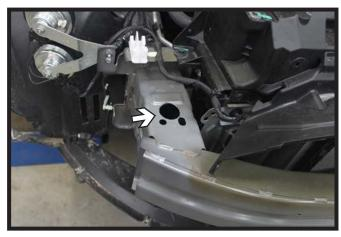
Using a 1-1/4" hole saw, drill an access hole on top of the bumper as shown. Do this on both sides of the vehicle.
