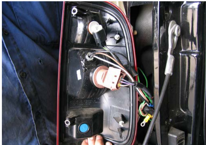
Possible location for the Bulb and Socket Wiring Kit (BX8869)
