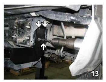
13. Using the baseplate as a template with the 13/32" drill bit, drill the three holes on the side.
