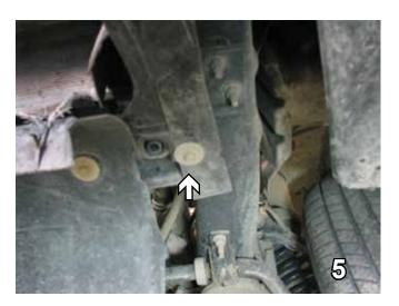
Using a 10MM socket, remove the screw from the lower black panel located forward of front tires and below air dam. Do this to both sides of the vehicle. Set screws aside to be reinstalled later.
