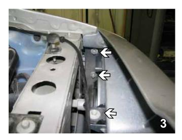
Using the 11MM socket, remove three metric hex nuts from both blinker assemblies, located just behind the head light area. Pull to the side, unplug and set aside. Do this to both sides of the vehicle.
