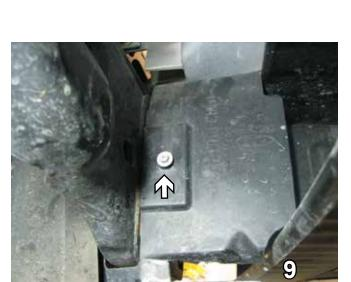
9. Using a 7MM socket, remove one metric screw on the air dam just behind the metal bumper. Do this to both sides.
