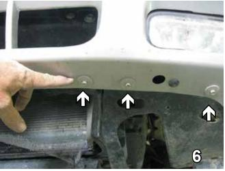
6. Using an 8MM socket, remove the eight screws with washers on the underside of the bumper fascia. Pull the fascia straight out to remove it. Do this to both sides of the vehicle. Set fascia and screws carefully aside to be reinstalled later.
