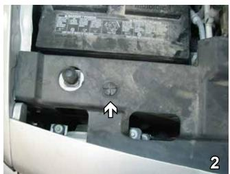
Unscrew three pins from the black plastic on the top edge of the fascia. Lift up and set plastic and pins aside to be reinstalled later.
