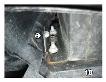
Remove the Christmas tree push pin from the air dam. Do this to both sides. Set pin aside to reinstall later.
