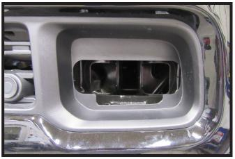
Remove baseplate. Using a utility knife trim the marked plastic area. Do this on both sides of the vehicle.
