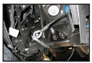
7. Attach the permanent baseplate safety cables to the provided convenience link on the baseplate. The photo above shows the recommended installation of the cables to frame of vehicle. Additional options may interfere with suggested mounting; in this case, secure the cables to a solid piece of the frame as described in the General Information sheet. Be sure the safety cables do not rub against any hoses or moving parts. Do this on **BOTH** sides of the vehicle.
