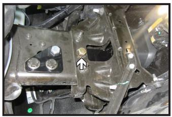
5. Slide baseplate into place. Insert one (1) 5/8" x 3-1/2" bolt into the existing hole. Tighten fully. Do this on both sides of the vehicle.
