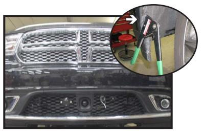
14. Hold the fascia as close to its original position, mark and trim the fascia around the convenience links and attachment tabs. Reinstall the fascia. Using the rivet gun, replace the rivets in each wheel well.
