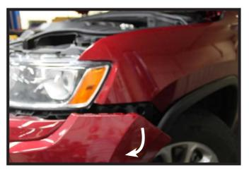
5. Pull the top corners of the fascia out releasing the clips behind, continue working inward towards the grille releasing the clips under the headlights. Pull the fascia forwards disconnecting all electrical connections and set the fascia aside.
