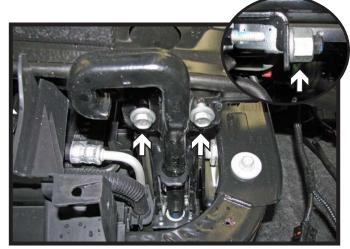
7. **Models equipped with tow hooks:** Using a 16MM socket, remove the two (2) bolts from the front side. Then using a 30MM socket or wrench, remove the nut from the backside of the tow hook. Remove the tow hook from the vehicle. Do this on both sides of the vehicle.
