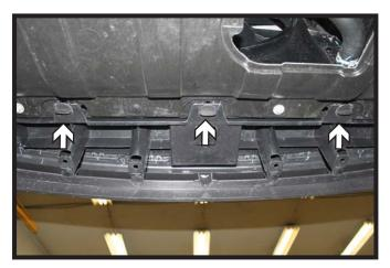
3. On the underside of the fascia, turn the three (3) locking knobs 90° to release.
