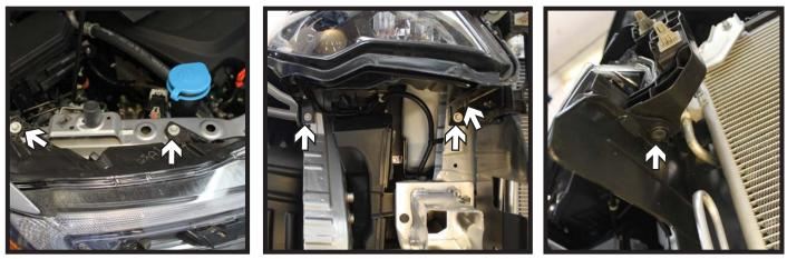
9. Using a 10MM socket, remove the five (5) screws from passenger side headlight assembly. There are two (2) on top, two (2) on the lower face and one (1) on the underside (left & middle). Next to the radiator remove the push pin as shown (right).
