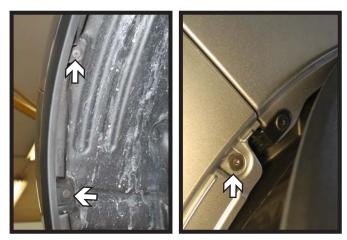
4. Using a phillips screwdriver, remove the three (3) screws from the edge of the wheel well (left). The upper two screws are shown the third screw is below.
