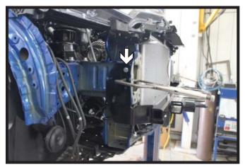
9. Position the baseplate onto the frame so it is touching the top and front frame lips. Level and securely clamp the baseplate. Using a 3/8" drill bit, drill the top front hole thru the frame. Install a 3/8"-16 x 1-1/4" bolt into the hole with a 3/8" lock washer and nut on the inside of the frame. Do this on both sides of the vehicle. Fully tighten all hardware.
