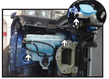
8. On the passenger side, remove the push pin from the washer reservoir neck (inset). Using a 10MM socket, remove the two (2) screws from the reservoir. Disconnect/plug all lines and set the reservoir aside.
