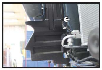
5. Trim off the plastic shrouding flush with the bottom side of the bumper. Do this on both sides of the vehicle.
