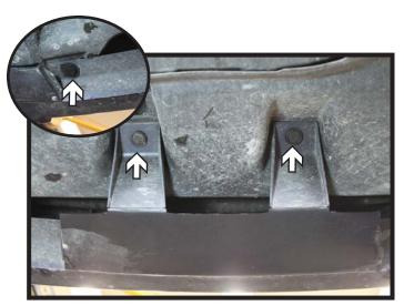
4. Remove the four (4) push pins from the underside of the fascia. There are two (2) in the center of the fascia and one (1) on either side of the center pins.
