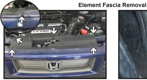
1. Remove the five (5) push pins from the fascia cover and set aside. Then remove the seven (7) push pins from the top edge of the fascia (inset).
