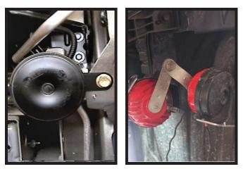
Models with Horns on DS/PS: Using a 13MM socket, loosen the bolt and turn the horn assembly outwards (left). Do this on both sides of the vehicle.
