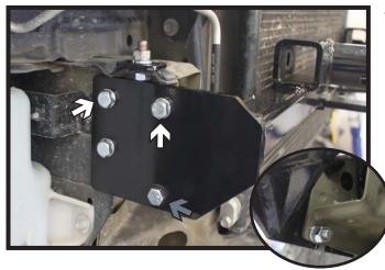
10. Using a 13/32" drill bit, drill the remaining holes thru the frame. Install 3/8"-16 x 1-1/2" bolts and lock washers into the top holes with a 3/8" nut plates on the inside of the frame. On the lower front hole install a 3/8"-16 x 1" bolt with a 3/8" lock washer and hex nut on the inside of the frame. Fully tighten all hardware. Do this on both sides of the vehicle.
