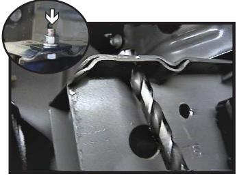
Using a 13/32" drill bit, drill a hole thru both frame layers as shown. Install a 3/8"-16 x 1" bolt from the underside thru the frame and install the support plate, a 3/8" lock washer and hex nut on the topside. Fully tighten the hardware. Do this on both sides of the vehicle.
