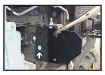
Position the baseplate onto the frame. Push the baseplate back to the sensor and approximately a 1/4" down from the frame flange. Level and securely clamp to the frame. Insure the tabs come thru the fascia properly.
