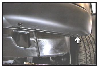
Using a 10MM socket, remove two (2) bolts from the bottom of edge of the fascia, just forward of the front tires. Remove two (2) push pins from the lower edge of the fascia. Do this to both sides of the vehicle.
