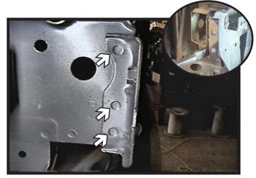
8. Using a 13/32" drill bit, drill the factory spot welds enough to release the flange from the frame. **DO NOT** drill thru the frame. Using a flat chisel separate the flange from the frame. Do this on both sides of the vehicle.
