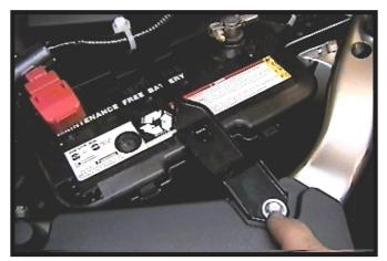
1. Using a 10MM socket, remove the metric bolt from the battery hold down strap.
