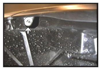
4. Using a 8MM socket, remove the bolt on the upper fascia corner. Do this to both sides of the vehicle. Pull the fascia forward and set carefully aside.
