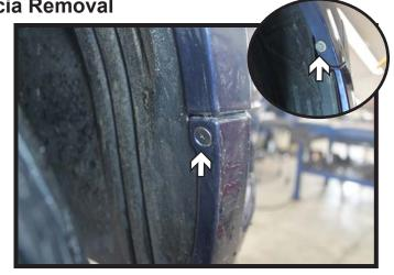
2. Using a Phillips screwdriver, remove the screw from the lower edge of the wheel well. Continue up along the edge of the wheel well and remove the upper screw (inset). Do this on both sides of the vehicle.
