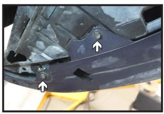
Using a 10MM socket, remove the four (4) screws from the corners of the fascia. There are two (2) on each side.
