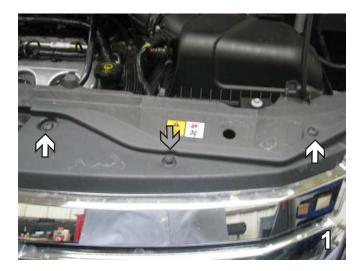
Using a Phillips screwdriver, remove two plastic Phillips push pins (see white arrows) and then using a 10MM socket, remove one bolt (see grey arrow) from the flat plastic piece on top. Do this to both sides of the vehicle. Set bolts and push pins aside to be reinstalled later.
