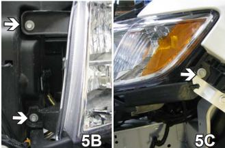
5. Using a 10MM socket, remove four bolts from the headlight assembly. Remove headlight by pulling it forward and disconnecting the electrical connections. Do this to both sides of the vehicle. Set headlight assemblies and bolts aside to be reinstalled later.
