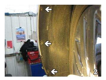
Using a 5.5MM socket, remove three bolts just forward of the front tire on the wheel well. Do this to both sides of the vehicle. Set bolts aside to be reinstalled later.
