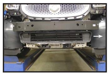
6. Slide the shroud towards the driver side and remove from the vehicle. The shroud will not be reinstalled.
