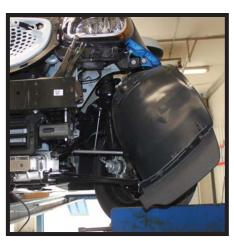
8. Turn the front wheels towards the driver side. In the wheel well, unfasten the plastic screw located along the frame (left). Remove the large push pin located by the fascia/fender joint (middle). Pull the wheel well liner away from the vehicle to access the frame for baseplate installation (right).
