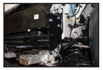
9. On the driver side, using a 18MM socket, remove the existing bolt on the underside of the frame. Reinstall the bolt with the baseplate and fully tighten (left). Clamp the side plate to the frame and drill the three (3) holes in the baseplate thru the bumper with a 3/8" drill bit. Install the 3/8" hardware into the holes and fully tighten all hardware (right).
