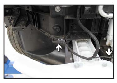
Remove the temperature sensor from bumper (right) then unhook clip from frame (left) and set aside.
