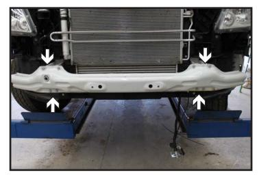
11. Remove the eight (8) bolts using a 13mm socket to remove bumper from frame.
