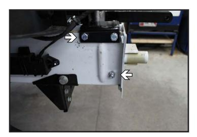
15. After upper front bolts are tightened down continue drilling upper back and lower front holes. In upper back hole (top) use 3/8"x4" bolt, 3/8" lockwasher and 3/8"-16 whiz nut with nut on inner side of frame. On front lower hole (bottom) use 3/8"x4" bolt and nylon lock nut with nut on outer side of frame.
