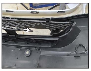
17. Hold front facia up to frame and mark to cut out for clearance around baseplate. After cutting sufficent amount for clearance, reattach facia to vehicle.
