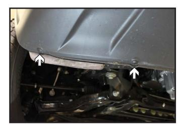
At the front of vehicle on the underside of facia using a straight screwdriver, turn the two (2) facia pins 90 degrees to unlock and remove. Both driver and passenger sides.
