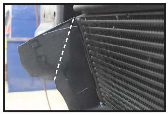
2013 Models: Trim the lower radiator shroud as shown for D-Link clearance on the baseplate. Do this on both sides of the vehicle.
