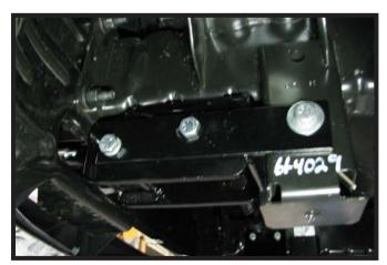
11. On the outer frame bolts, install 1/2" lock washers onto the front two (2) bolts. Then a 1/2" flat washer onto the rear hole. Fully tighten all bolts. Repeat on the other side of the vehicle.
