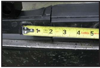
14. On the lower air dam, measure 2" out from the second hole and cut apart. Do this on both sides. Reattach the lower air dam, the plastic bumper and reconnect the plug. If your vehicle is equipped with tow hooks, you will not need to trim the air dam.
