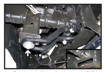
4. If equipped with tow hooks, use a 18MM socket to remove the lower bolt (white) and the two (2) upper nuts on either side of the frame (gray). Remove the tow hook and reinstall the upper nuts back onto the frame. Repeat on the other side of the vehicle.
