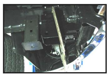
5. Tip the baseplate at an angle, then slide it into the opening and up to the frame. Clamp the baseplate to the frame.
