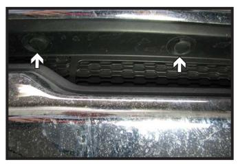
2009-12 Models: Remove the six (6) push pins along the front plastic insert and remove from the vehicle.
