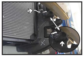
8. On the driver side, remove the temperature sensor from the shrouding (inset). Then trim off the lower section of the shrouding flush with the bottom of the bumper.
