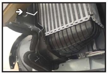
9. On the passenger side, trim the lower section of the shrouding off flush with the bottom of the bumper.
