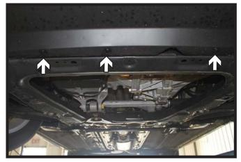
5. Remove the three (3) push pins from the underside of the fascia towards the center. Gently pry the fascia from the vehicle, disconnecting any electrical connections and set the fascia aside.
