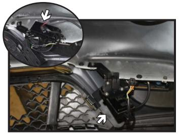
Nismo Only: On the backside of the fascia, unscrew the fog light box and flip upside down and reattach to the fascia as shown for baseplate clearance. Do this on both sides of the fascia.
