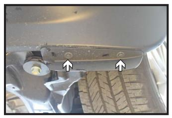
Using a 10MM socket, remove the four (4) screws from the underside of the fascia in front of the tire. There are two (2) on each side.
