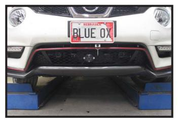
19. Hold the fascia as close to its original position, mark and trim the fascia around the convenience links and attachment tabs. Reinstall the washer reservoir using the supplied lower bolt. Reinstall the baffle and fascia.
