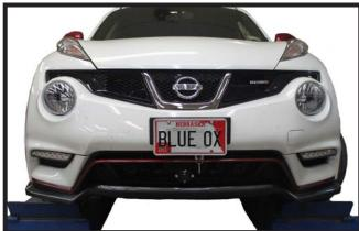
Reference your vehicle owner's manual for manufacturer's towing specifications. Attachment Tab Height: 16"
