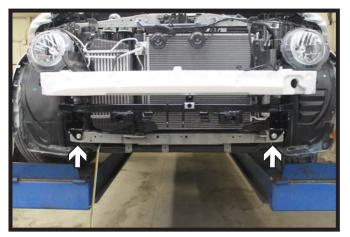
Using a 1-1/4" hole saw, drill an access hole behind the flange as shown (gray). Do this on both sides of the vehicle.
