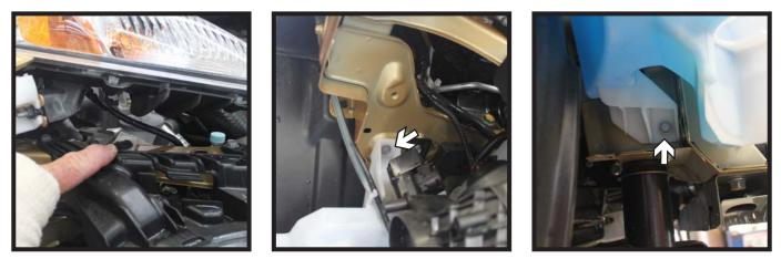
7. On the passenger side, remove the push pin from the washer reservoir just below the blinker (left). Using a 10MM socket, remove the upper screw (middle) and lower screw (right) from washer reservoir. Disconnect all lines and set reservoir aside.
