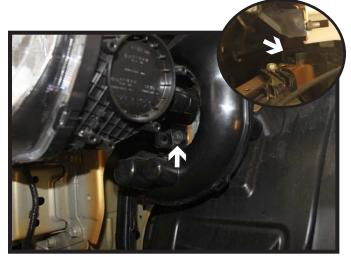
On the driver side, using a 10MM socket, remove the screw from the lower section of the baffle. Remove the push pin from the upper section just below the blinker (inset). Set the baffle aside.
