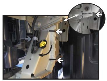
10. Cut two (2) slits into the frame webbing as shown. Bend this section of webbing forward flat against the frame. Unclip the wiring harness from the face of the frame and secure out of the way. Do this on both sides of the vehicle.
