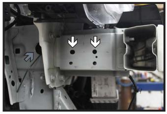
13. Using a 1/2" drill bit, ream out the two(2) top existing holes for bolt clearance (white).
