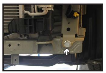
11. Using a 17MM socket, remove the two (2) bolts from the lower frame. There is one (1) on each side.
