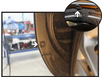
2. In the wheel well, remove the two (2) push pins. There is one (1) on the lower edge and one (1) on the upper edge (inset). Do this on both sides of the vehicle.
