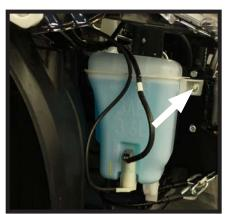
10. Reconnect the windshield wiper fluid reservoir using the existing fasteners except
