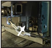
the baseplate. The photo above shows the recommended installation of the cables to frame of vehicle. Additional options may interfere with suggested mounting; in this case, secure the cables to a solid piece of the frame as described in the instructions included with the permanent baseplate safety cables. Be sure the safety cables do not rub against any hoses or moving parts. Do this on **BOTH** sides of the vehicle.
