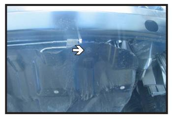
Using the 10MM socket, remove the two (2) bolts from the belly pan that bolt into the bottom of the metal bumper.
