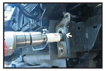
13. Using a 1-1/4" holesaw, drill a hole as shown in the driver's side frame that is connected with the existing hole for nut plate access.
