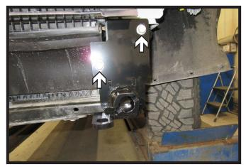
11. Start the two (2) existing 10MM bolts into the front holes. May need to lift baseplate for holes to line up. Tighten bolts but do not use Loctite Red at this time. Do this on both sides of the vehicle.
