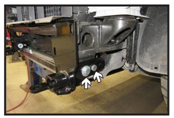
Slide baseplate into place and insert two (2) 1/2" x 3-1/2" bolts into the side holes. Use a flat washer with front bolt. Do not install nuts at this time.
