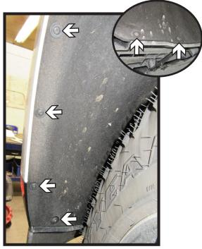
4. Using a T15 Torx, remove the six (6) bolts from along the edge of the wheel well. Do this on both sides of the vehicle.
