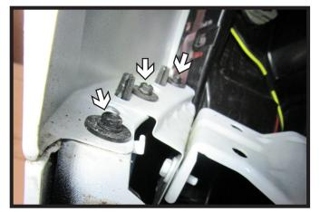
6. Pull back the wheel well liner and using a 7MM socket, remove the three (3) bolts from the fascia joint. Do this on both sides of the vehicle.
