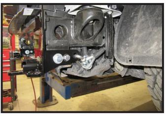
13. Before reinstalling bumper, attach the permanent baseplate safety cables to the provided convenience link on the baseplate. The photo above shows the recommended installation of the cables to frame of vehicle. Additional options may interfere with suggested mounting; in this case, secure the cables to a solid piece of the frame as described in the General Information sheet. Be sure the safety cables do not rub against any hoses or moving parts. Do this on **BOTH** sides of the vehicle.
