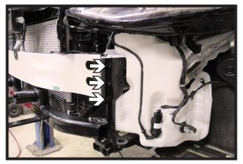
21. Start the front three (3) 3/8" bolts with hardware. Do this on both sides of the vehicle.
