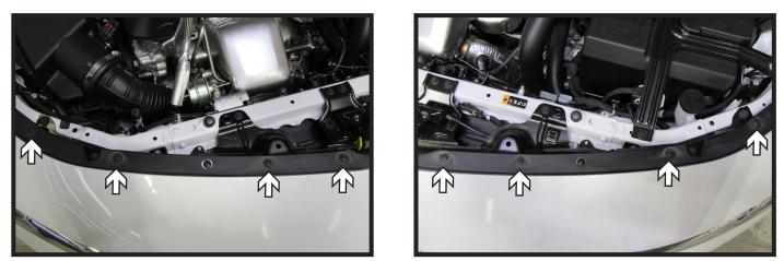
Using a T15 Torx, remove the eight (8) screws from the top edge of the fascia. There are four (4) on each side. Remove the black plastic cover from each side of the vehicle.
