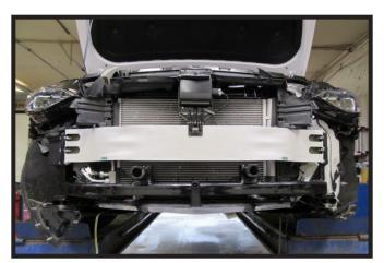
24. Reinstall plastic shield, air dam, and headlights. Reconnect all electrical connections.
