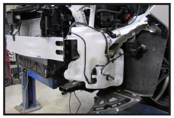
19. Reinstall the windshield washer fluid reservoir on the driver side of the vehicle.
