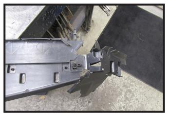
15. Using a utility knife, cut the sides off of the plastic shielding as shown to allow clearance for baseplate.
