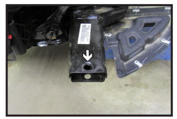
13. Using a 1/2" drill bit, drill out the existing hole on the frame extension. Do this on both sides of the vehicle.
