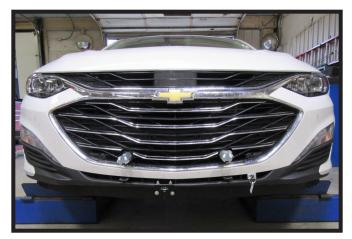
25. Hold the fascia as close to its original position, mark and trim the fascia around the convenience links and attachment tabs. Reinstall the fascia.
