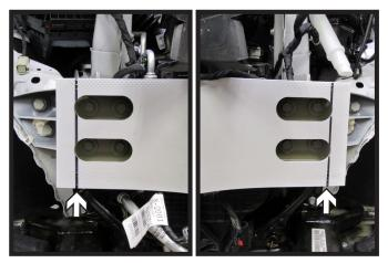
11. Using a reciprocating saw, trim the bumper as indicated so it is flush with the frame. Do this on both sides of the vehicle.
