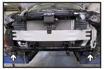
20. Set the baseplate in place and start the 1/2" bolt with hardware and insert on each side of the baseplate.
