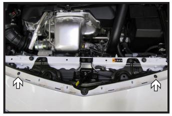
2. Using a T15 Torx, remove the two (2) screws from the top edge of the fascia. There is one (1) on each side.
