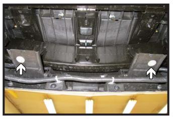
6. All Tahoe/Suburban Models: Using a 10MM socket, remove the two (2) remaining screws from the underside of the fascia.
