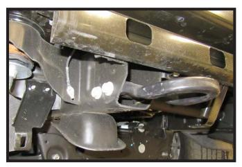
12a. **All Tahoe/Suburban Models:** Using a 18MM socket remove the six (6) bolts, three (3) on each side, attaching the tow hooks and remove tow hooks. Do this on both sides of the vehicle.
