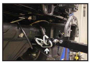
16. All Models: Attach the permanent baseplate safety cables to the provided convenience link on the baseplate. The photo above shows the recommended installation of the cables to frame of vehicle. Additional options may interfere with suggested mounting; in this case, secure the cables to a solid piece of the frame as described in the General Information sheet. Be sure the safety cables do not rub against any hoses or moving parts. Do this on BOTH sides of the vehicle.
