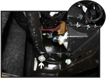
9. All Silverado/Sierra Models: Using a 15MM socket, remove the bolt from the bumper reinforcement bar. Do this on both sides of the vehicle. Disconnect the running lights/electrical connections (gray).
