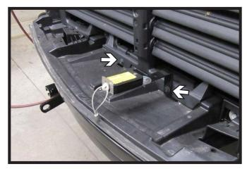
19. Optional Tahoe/Suburban Models: Using either existing bolt attach the brakeaway bracket. Then use a 1/4" bolt to attach the brakeaway switch to the bracket.
