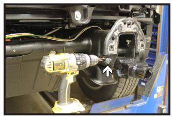
14. **All Models:** Insert the front 1/2" bolt and start the bottom 1/2" bolt with step washer, do this on both sides of the vehicle. Do not fully tighten the bolts. Note: The bottom frame hole may need to be reamed out to align with the slot.
