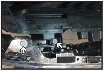
10. **All Silverado/Sierra Models:** Using a 18MM socket, remove the four (4) bolts from the top of the bumper. There are two (2) on each side. Set the bumper aside.
