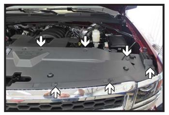
1. **All Models:** Remove the twelve (12) push pins from the shroud cover. There are six (6) on each side. Set the cover aside.
