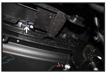
7b. Sierra 1500 Models: Unsnap the six(6) tabs from the backside of the fascia.Remove the fascia from the vehicle and set aside.
