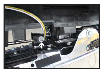
18. All Silverado/Sierra Models: Reinstall the cover plates and bumper onto the vehicle. Install the top outer bolts, then push in on the bottom of the bumper to line up the inner bottom bolts. Clamp the bumper when the hole is lined up and reinstall the lower bolts. Continue to reinstall the bumper bar bolts and reconnecting the electrical connections on the underside of the bumper.
