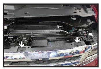
2b. **All Silverado/Sierra Models:** Using a 10MM socket, remove the four (4) screws from the top edge of the grille. There are two (2) on each side.
