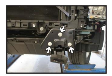
11. **All Silverado/Sierra Models:** Using a 15MM socket, remove the three (3) bolts from the cover plate. Do this on both sides of the vehicle.
