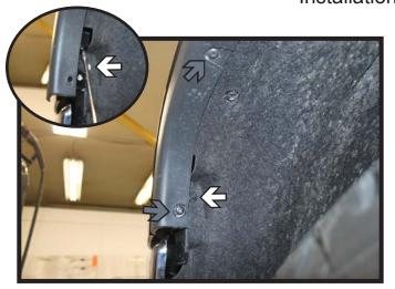
3b. **Sierra 1500 Models:** Using a 7MM socket, remove the screw from the wheel well (white). Using a T15 Torx, remove the screws (gray).
