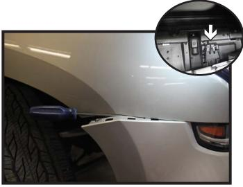
7a. All Tahoe/Suburban Models: Gently pry the clips of the corners of the fascia loose from the fender. Behind the grille towards the base, pop loose the two (2) clips. Remove the fascia from the vehicle and set aside.
