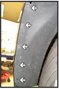
3a. **All Tahoe/Suburban Models:** Using a 7MM socket, remove the screws from the edge of the wheel well. Do this on both sides of the vehicle. Quantity of screws vary per model.
