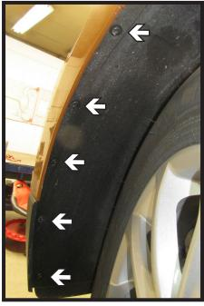
Using a T15 Torx, remove the five (5) bolts from along the edge of the wheel well. Do this on both sides of the vehicle.
