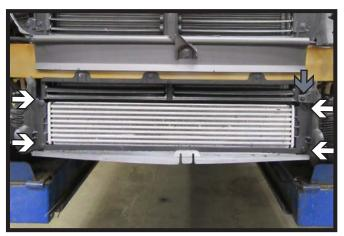
8. Remove the temperature sensor (gray) and then remove the four (4) push pins (white) holding the plastic piece on the front of the grill. Set aside to be trimmed and reinstalled later.
