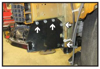
12. Drill the remaining four (4) holes on each side of the baseplate and install the 3/8" hardware.
