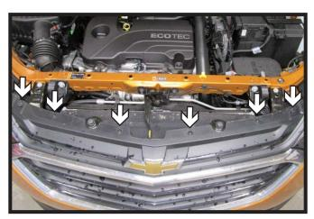
1. Using a T15 Torx, remove the six (6) screws from the top edge of the fascia. There are three (3) on each side.
