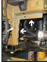
Use a hammer to tap the metal frame pieces inward slightly, about 1/8", to allow clearance for baseplate. Do this on both sides of the vehicle.
