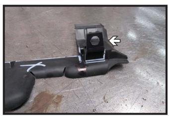
14. Remove the temperature sensor holder from the removed driver side plastic piece to be reinstalled on the vehicle.
