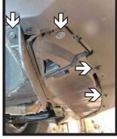
Using a 7MM socket, remove the eight (8) bolts from the underside of the fascia, four (4) on each side.
