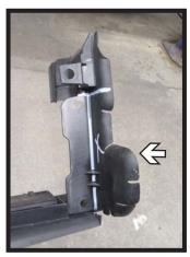
13. Using a utility knife, trim the indicated areas from the plastic piece before reinstalling to the front of the grill using existing push pins.
