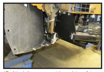
17. Attach the permanent baseplate safety cables to the provided convenience link on the baseplate. The photo above shows the recommended installation of the cables to frame of vehicle. Additional options may interfere with suggested mounting; in this case, secure the cables to a solid piece of the frame as described in the General Information sheet. Be sure the safety cables do not rub against any hoses or moving parts. Do this on **BOTH** sides of the vehicle.
