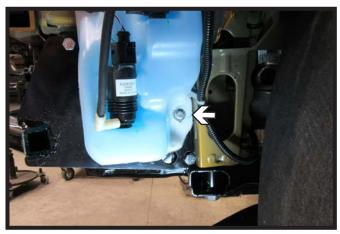
16. Reinstall the windshield washer fluid reservoir using existing hard ware except for the indicated bolt, use the 6MM bolt and 1/4" flat washer provided to attach to the baseplate. Reconnect all lines. Reinstall driver side headlight.
