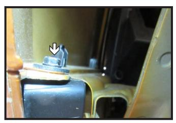
Pull back the wheel well liner. Then using a 7MM socket, remove the bolt from inside the wheel well. Do this for both sides of the vehicle.
