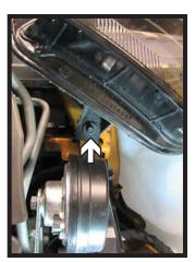
6. Using a 7MM socket remove the four (4) bolts attaching the driver side head light. Remove and set aside to be reinstalled later.
