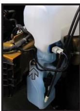
7. Using a 10MM socket, remove the three (3) bolts (white arrows) and one (1) nut (gray arrow) holding the windshield washer reservoir. Unplug all lines and set aside to be reinstalled later.
