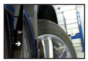
3. Carefully remove the plastic panel from the both sides of the vehicle.
