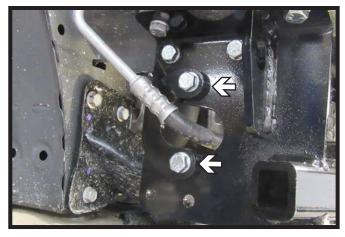
On the passenger side, attach the reinforcement brace around the line. Install with the provided 3/8" hardware.
