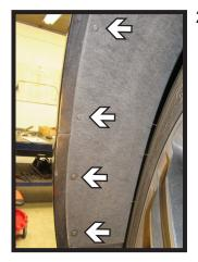
2. Using a T15 Torx, remove the four (4) screws from the wheel well in front of the tire. Do this for both sides of the vehicle.
