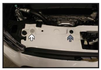
Using a 10MM socket, remove the screw from the top edge of the fascia (white). Then remove the push pin inwards toward the hood latch (gray). Do this on both sides of the vehicle.
