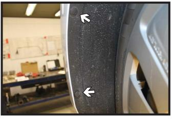
2. Remove the two (2) push pins from along the edge of the wheel well. Do this on both sides of the vehicle.
