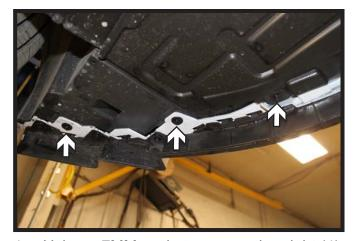
4. Using a 7MM socket, remove the eight (4) screws from the underside of the fascia. There are three (3) on each side and two (2) in the center.
