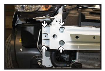
7. Remove the four (4) push pins from the top of the bumper.
