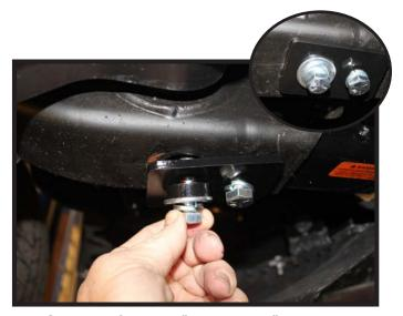
4. Start the front 1/2"-13 x 1-1/2" bolt with lock washer and spacer plate into the baseplate to align it with the frame. Install the rear 1/2"-13 x 1-1/2" bolt with lock, flat washer and spacer sleeve into the baseplate. Fully tighten all hardware. Do this on both sides of the vehicle.
