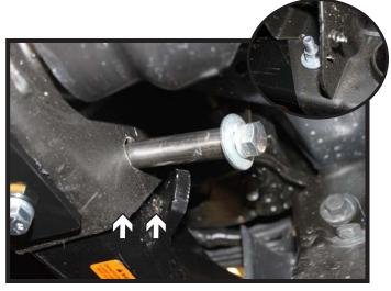
5. Install the 1/2"-13 x 5" bolt with lock, flat washer and frame sleeve into the inside frame hole. Install a 1/2" flat washer and lock nut onto the bolt on the outside of the frame (inset). Fully tighten all hardware. Do this on both sides of the vehicle.
